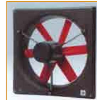
The POULTEC range of multi-speed fans covers all the possible uses in modern farms, with different motors operating on single or three-phase currents and for 50 or 60 Hz. Operating on speeds varying from 800 to 3200 RPM, and powers of 120 to 1800 W according to motor and current type.
